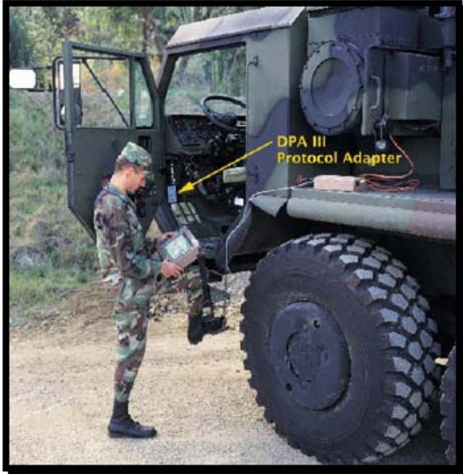
Figure 4: Heavy Vehicle Scan Tool System
