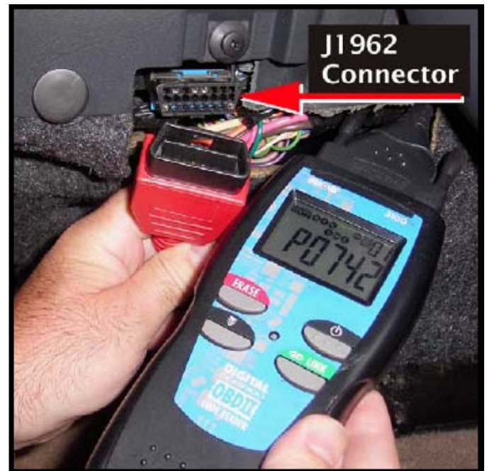
Figure 3: OBDII Scan Tool
