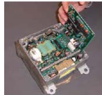
Figure 2: ECM - Example Electronic Control Module
