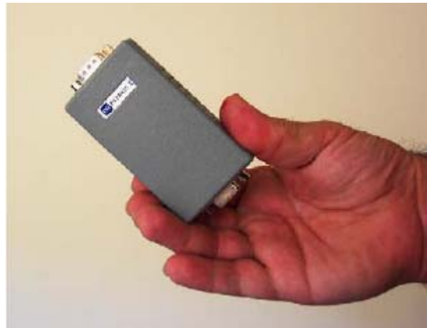
Figure 5: J2534 Pass Through Adapter
